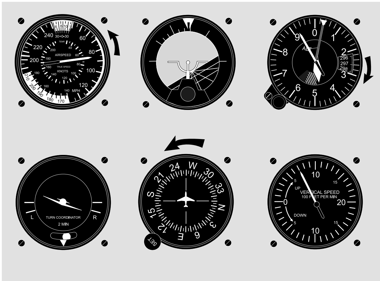
Figure 147. – Instrument Sequence (Unusual Attitude).
